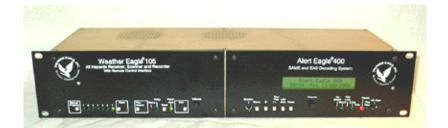
The AlertEagle®400 (AE400) is a high performance, patented, diagnostic EAS/SAME decoder. The AE400 system includes the Weather Eagle 105 radio receiver and the AE400 decoder. This system translates EAS/SAME encoded messages from NOAA's National Weather Service into readable text and relays that text by LAN/WAN and Internet to printers, email and pagers. The system is designed in a modular fashion so that parts of the system can be added as your budget permits.
